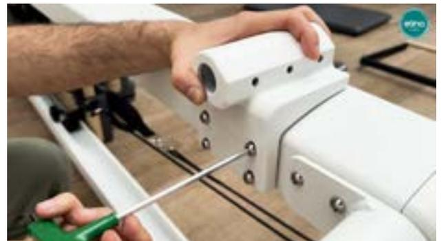
We begin by placing the metal parts supporting the tower on the structure. We must place the washer towards the inside of the reformer, in the long part of it.
