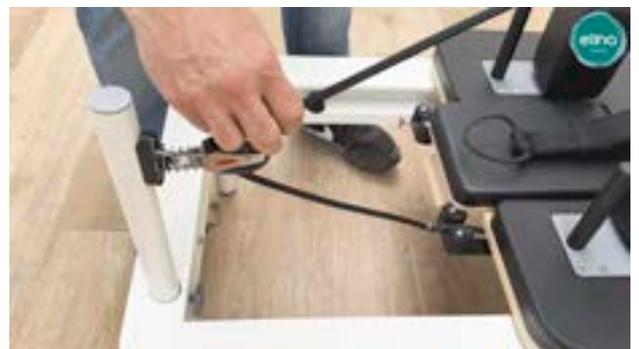
We insert the ropes into the pulleys, starting by passing the free end through the pulley. Next, we pass the rope through the designated set screws to regulate the length of the rope.
