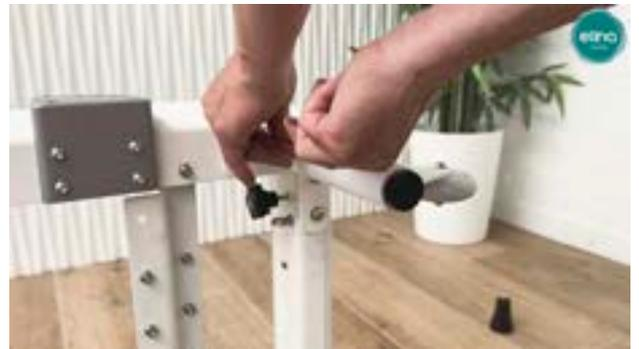
The legs with wheels are placed on the bottom of the reformer, making sure that the wheels are facing outwards. Secure the legs in the same way.
