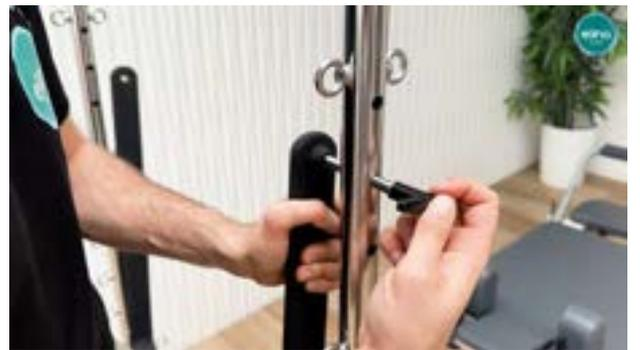
We place the push bar on the tower, inserting the fastening anchors from the outside.
