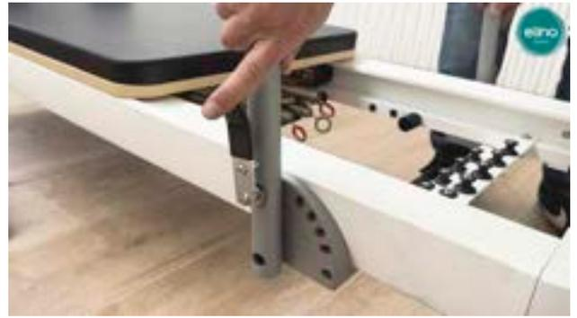
To place the footbar, press the position adjustment tab and place it in the desired position.
