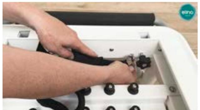
We attach the foot strap to the internal attachment point of the reformer.
