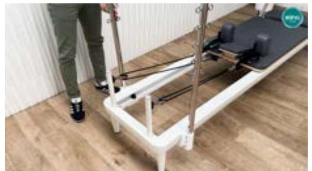
We should not tighten the fastening screws too much in order to facilitate the placement of the tower posts. Repeat the process on both sides.
